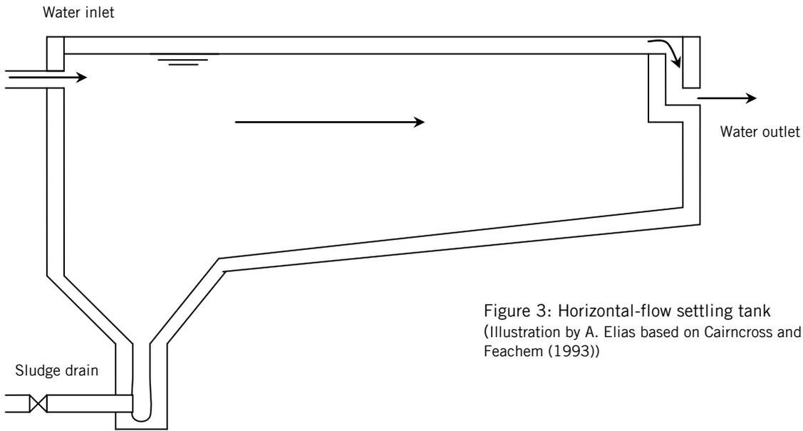
Figure 3: Horizontal-flow settling tank (Illustration by A. Elias based on Cairncross and Feachem (1993))
