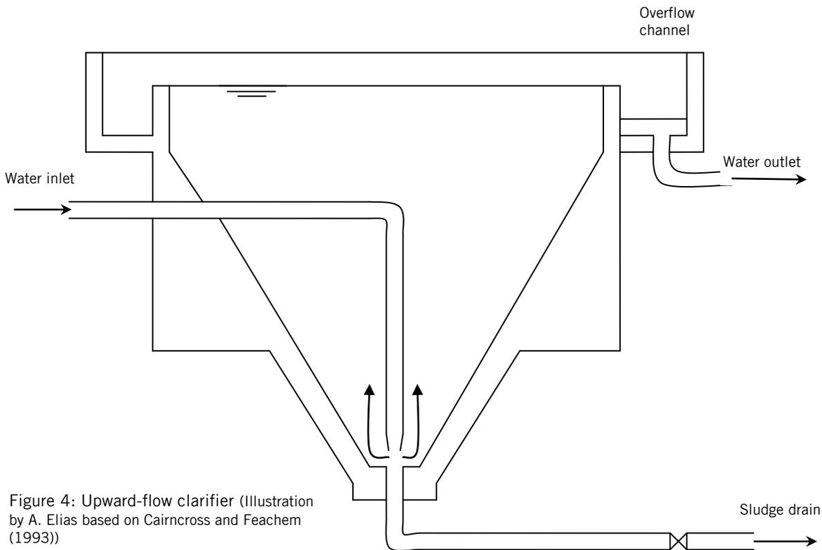
Figure 4: Upward-flow clarifier (Illustration by A. Elias based on Cairncross and Feachem (1993))
