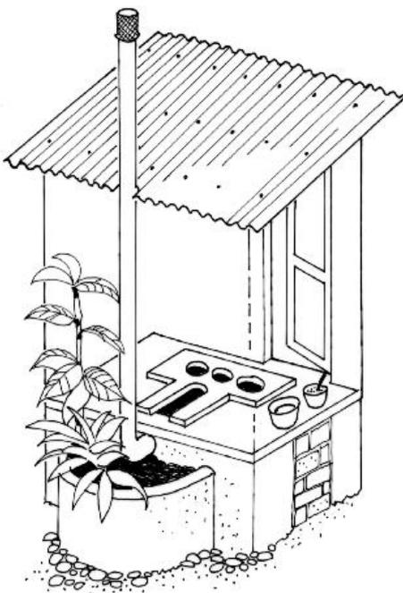
In areas where water is used for anal cleansing there is a risk of the contents of dehydrating toilets becoming too wet and therefore not operating properly. The Kerala double vault toilet (figure 3) contains a trough over which to wash to prevent the contamination of the drying waste. In this system the water is collected together with the urine.
