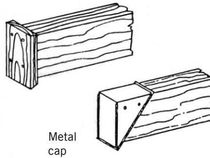
Figure 4: Simple ways of protecting end grain
