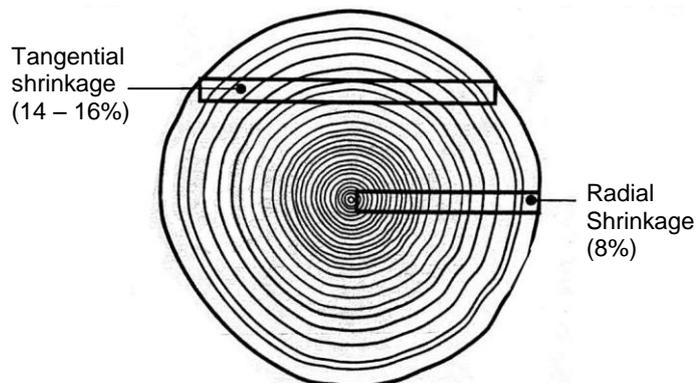
Figure 3: Timber shrinkage
